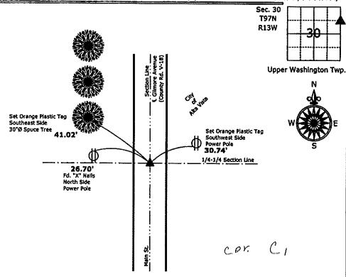
Southeast Corner NE 1/4-NE 1/4Section 30-97-13 Set 5/8\*Ø rebar w/2\*Ø aluminum cap PLS 19211, punched cap for position
