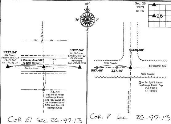
1.) Northeast Corner NW 1/4-NW 1/4 Section 26-97-13 Set Survey Mark Nail with Stainless Steel Washer PLS 19211
