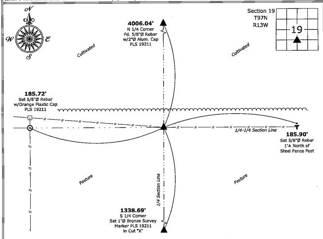
Northwest Corner of the SW 1/4 - SE 1/4 of Section 19-97-13 Set 5/8"Ø Rebar w/2"Ø Aluminum Cap PLS 19211
