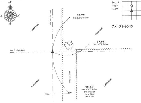
Center of Section 9-96-13 Set 5/8"Ø Rebar w/2"Ø Aluminum Cap PLS 19211 (Buried 18" Deep)
