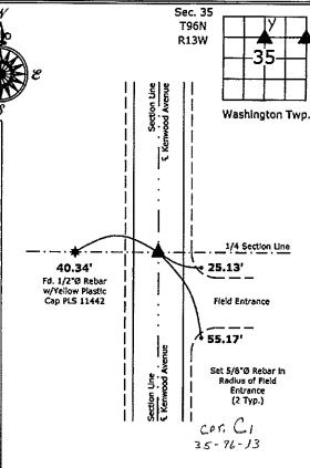
2.) NE Corner SE 1/4-NE 1/4 Section 35-96-13 Set Survey Mark Nail w/ Stainless Steel Washer PLS 15525
