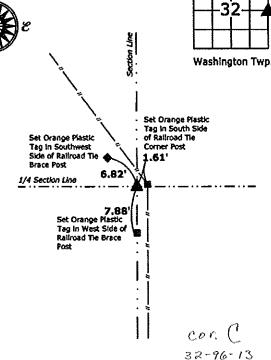
2.) East 1/4 Corner Section 32-96-13 Set 5/8"Ø rebar w/2"Ø aluminum cap PLS 15525
