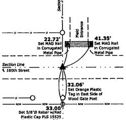
1.) Northeast Corner Section 32-96-13 Fd. 1/2°Ø rebar
