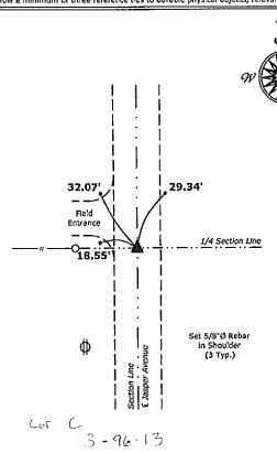
1.) West 1/4 Corner Section 2-96-13 Found 1/2"Ø rebar w/2"Ø aluminum cap PLS 7060
