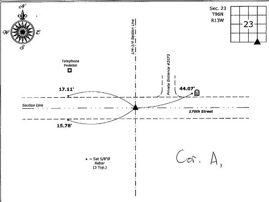
Southwest Corner SE 1/4 - SE 1/4 of Section 23-96-13 Set 5/8"Ø rebar w/2"Ø aluminum cap PLS 15525
