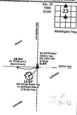
1.) Center of Section 23-96-13 Set 5/8\*Ø rebar w/2\*Ø aluminum cap PLS 19211
