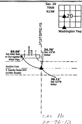
2.) Southwest Corner SE 1/4-SW 1/4 Section 20-96-13 Set 5/8\*Ø rebar w/2\*Ø aluminum cap PLS 15525
