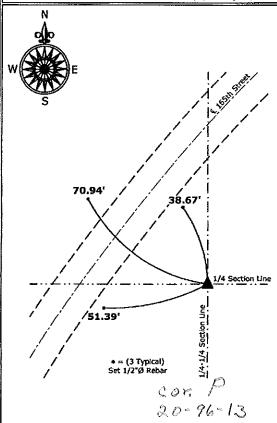
1.) Northwest Corner NE 1/4-SW 1/4 Section 20-96-13 Set 5/8"Ø rebar w/2"Ø aluminum cap PLS 15525
