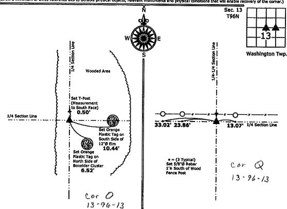
1.) Center of Section 13-96-13 Set 5/8°Ø rebar w/2°Ø aluminum cap PLS 15525
