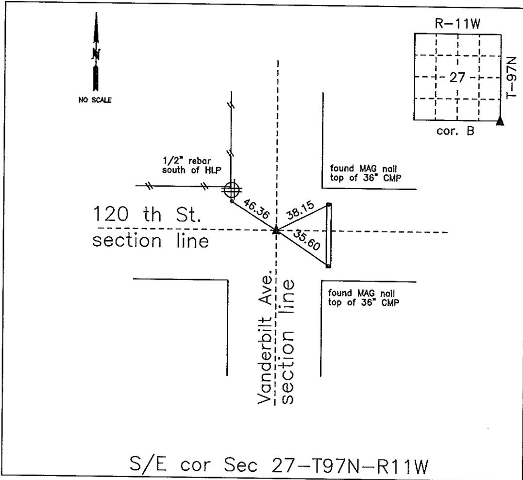
**MONUMENT DESCRIPTION AND NARRATIVE** Found iron pin in center of road in line with both roads north/south & east/west from county engineer ties. 3 ties were missing. Set 1 rebar w/caps south of power pole at n/w cor of intersection.
