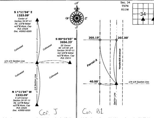
1.) Southwest Corner NW 1/4-SE 1/4 Section 34-97-11 Set 5/8"Ø rebar w/2"Ø aluminum cap PLS 19211
