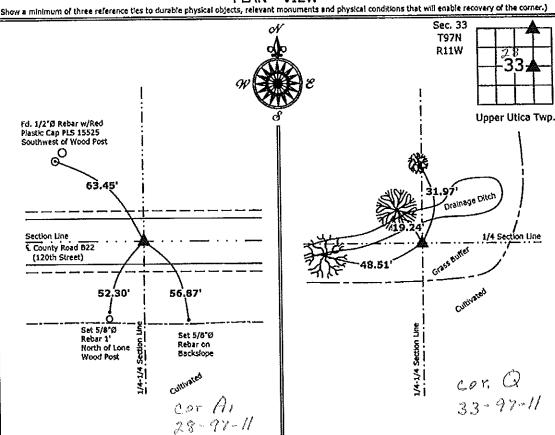
1.) Northeast Corner NW 1/4-NE 1/4 Section 33-97-11 Set Survey Mark Nail w/Stainless Steel Washer PLS 19211  Southeast Corner SW 1/4-NE 1/4 Section 33-97-11 Set 5/8\*Ø rebar w/2\*Ø Aluminum Cap PLS 19211
