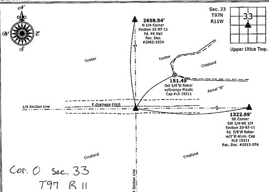
Center of Section 33-97-11 Set 5/8"Ø rebar w/2"Ø aluminum cap PLS 19211
