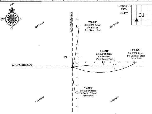
Southwest Corner of the NE 1/4 - SW 1/4 of Section 31-97-11 Set 5/8"Ø Rebar w/2"Ø Aluminum Cap PLS 19211
