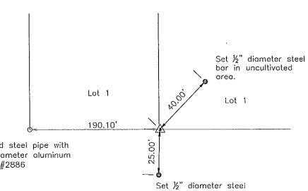
Found steel pipe with 1" diameter aluminum cap #2886
