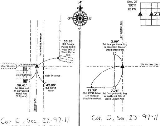
1.) West 1/4 Corner Section 23-97-11 Set 5/8"Ø rebar w/2"Ø aluminum cap PLS 19211 2.) Center of Section 23-97-11 Set 5/8"Ø rebar w/2"Ø aluminum cap PLS 19211
