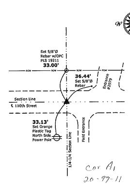
1.) Southwest Corner SE 1/4 SE 1/4 Section 20-97-11 Set 5/8"Ø rebar w/2"Ø aluminum cap PLS 19211
