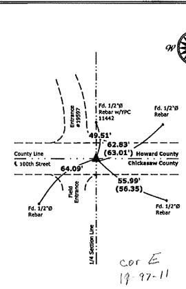
1.) North 1/4 Corner Section 19-97-11 Set Survey Mark Nail w/Stainless Steel Washer PLS 19211
