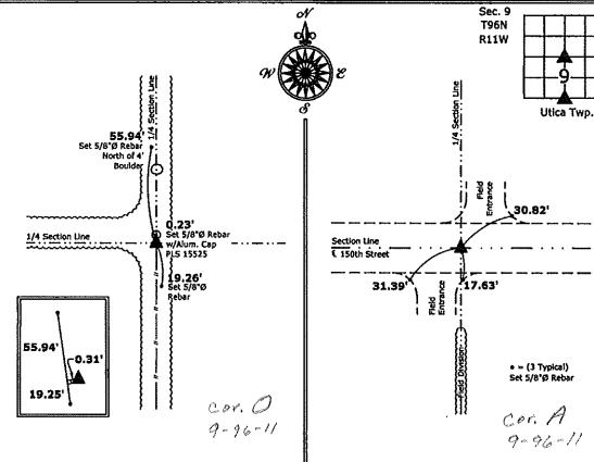
1.) Center of Section 9-96-11 Fd. 9" x 12" Granite Stone 2.) South 1/4 Corner Section 9-96-11 Set 5/8\*Ø rebar w/2\*Ø aluminum cap PLS 15525
