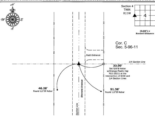
West 1/4 Corner of Section 4-96-11 Set 5/8"Ø Rebar w/2"Ø Aluminum Cap PLS 19211
