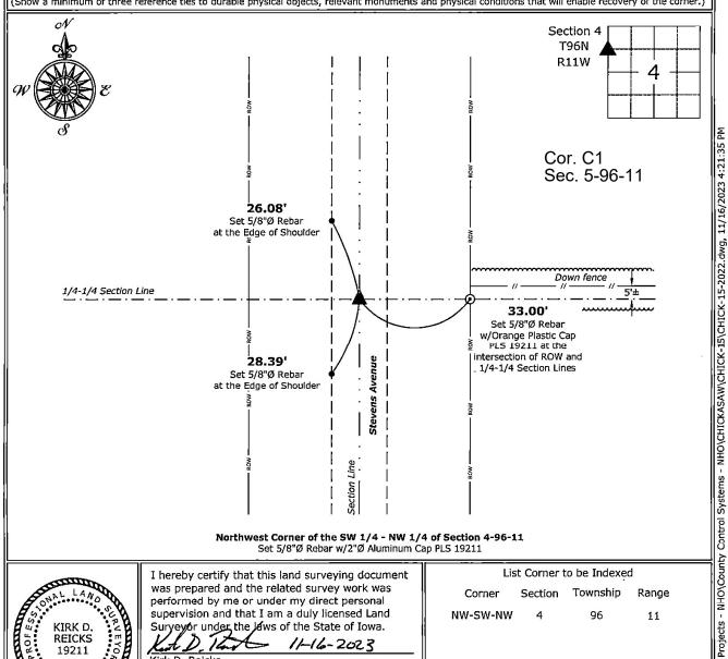
Northwest Corner of the SW 1/4 - NW 1/4 of Section 4-96-11 Set 5/8"Ø Rebar w/2"Ø Aluminum Cap PLS 19211
