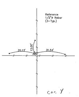
NW-SW-NE Corner Section 4 T96N R11W Set 1/2"ø rebar w/2"ø aluminum cap PLS 15525
