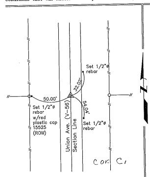
NE Corner SE 1/4-NE 1/4 Section 4 T96N R11W Set MAG nail w/SSW PLS 15525
