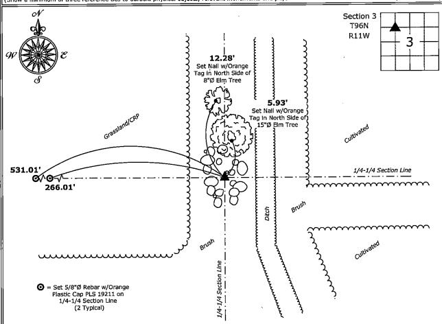
Northeast Corner of the SW 1/4 - NW 1/4 of Section 3-96-11 Set 5/8"Ø Rebar w/2"Ø Aluminum Cap PLS 19211
