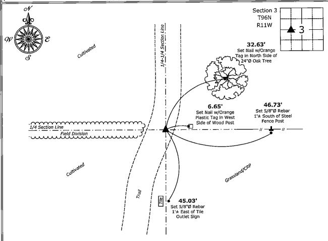
Southeast Corner of the SW 1/4 - NW 1/4 of Section 3-96-11 Set 5/8"Ø Rebar w/2"Ø Aluminum Cap PLS 19211
