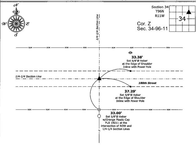
Northeast Corner of the SW 1/4 - NE 1/4 of Section 34-96-11 Set 5/8"Ø Rebar w/2"Ø Aluminum Cap PLS 19211
