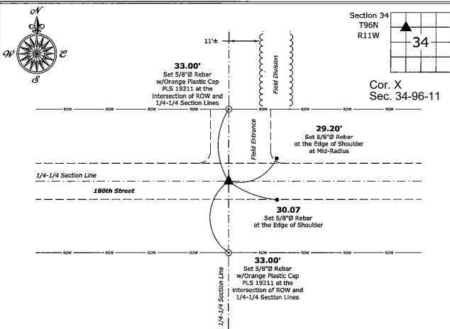
Southeast Corner of the NW 1/4 - NW 1/4 of Section 34-96-11 Set 5/8"Ø Rebar w/2"Ø Aluminum Cap PLS 19211
