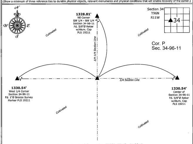
Southeast Corner of the SW 1/4 - NW 1/4 of Section 34-96-11 Set 5/8"Ø Rebar w/2"Ø Aluminum Cap PLS 19211 Buried 18"± deep
