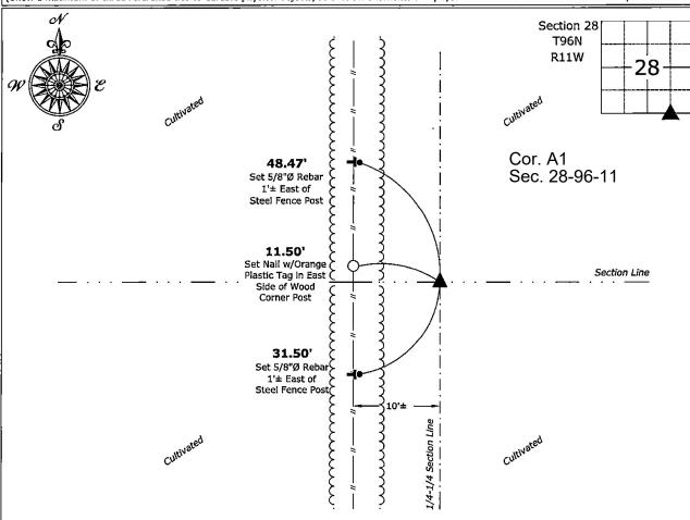
Southwest Corner of the SE 1/4 - SE 1/4 of Section 28-96-11 Set 5/8"Ø Rebar w/2"Ø Aluminum Cap PLS 19211
