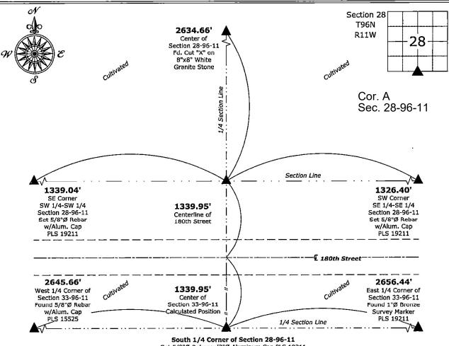
South 1/4 Corner of Section 28-96-11 Set 5/8"Ø Rebar w/2"Ø Aluminum Cap PLS 19211 Buried 18"± deep
