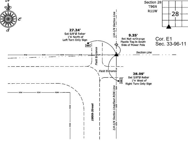
Southeast Corner of the SW 1/4 - SW 1/4 of Section 28-96-11 Set 5/8"Ø Rebar w/2"Ø Aluminum Cap PLS 19211
