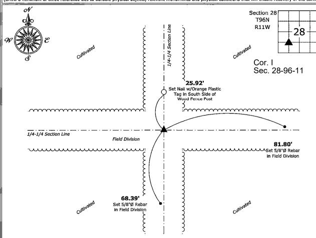
Northeast Corner of the SW 1/4 - SW 1/4 of Section 28-96-11 Set 5/8"Ø Rebar w/2"Ø Aluminum Cap PLS 19211
