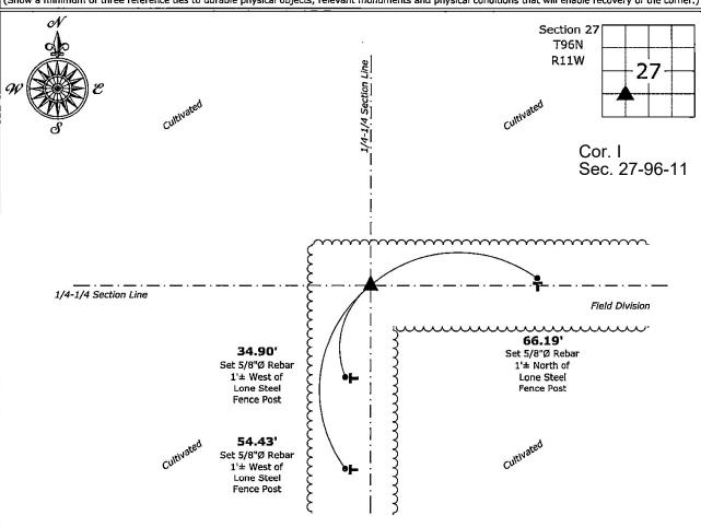
Northeast Corner of the SW 1/4 - SW 1/4 of Section 27-96-11 Set 5/8"Ø Rebar w/2"Ø Aluminum Cap PLS 19211
