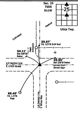
1.) North 1/4 Corner Section 25-96-11 Set 5/8"Ø rebar w/2"Ø aluminum cap PLS 19211
