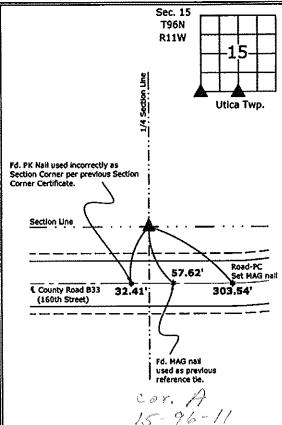
2.) South 1/4 Corner Section 15-96-11 Set 5/8"Ø rebar w/2"Ø aluminum cap PLS 19211
