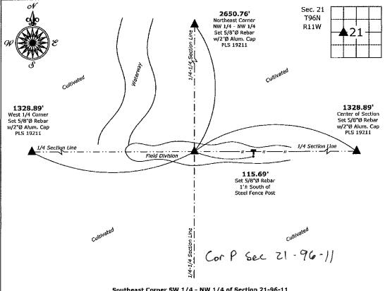
Southeast Corner SW 1/4 - NW 1/4 of Section 21-96-11 Set 5/8"Ø rebar w/2"Ø aluminum cap PLS 19211
