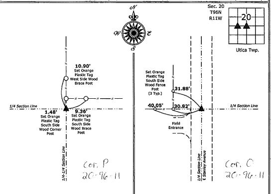
1.) Southwest Corner Se 1/4-NW 1/4 Section 20-96-11 Set 5/8\*Ø rebar w/2\*Ø aluminum cap PLS 19211 2.) Center of Section 20-96-11
