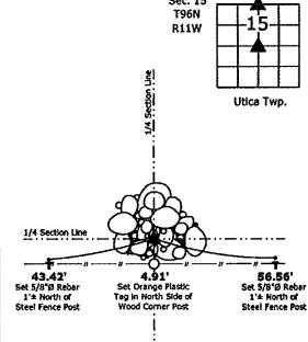
2.) Center of Section 15-96-11 Set 5/8"Ø rebar w/2"Ø aluminum cap PLS 19211
