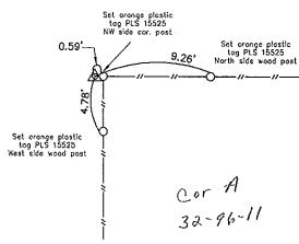
N 1/4 Corner Section 5 T95N R11W Set 1/2\*ø rebar w/2\*ø aluminum cap PLS 15525
