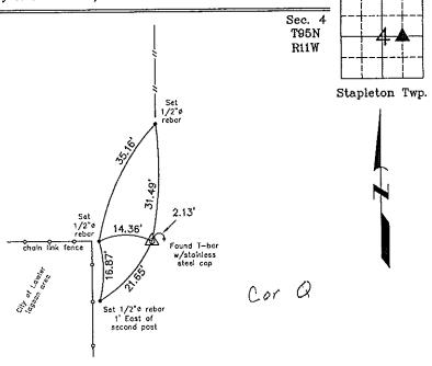
SW Corner SE 1/4 - NE 1/4 Section 4 T95N R11W Set 1/2"ø rebor w/2"ø aluminum cap PLS 15525
