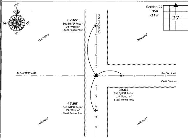
North 1/4 Corner of Section 27-95-11 Set 5/8"Ø Rebar w/2"Ø AlumInum Cap PLS 19211
