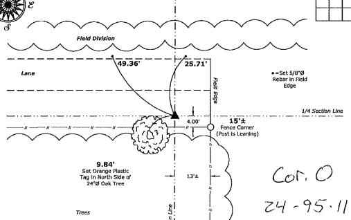
Center of Section 24-95-11 Set 5/8"Ø rebar w/2"Ø aluminum cap PLS 19211
