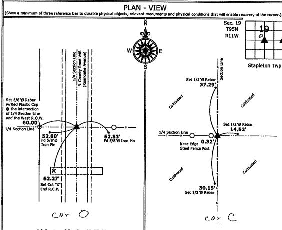
1.) Center of Section 19-95-11 Set Survey Mark Nail w/stainless steel washer PLS 15525
