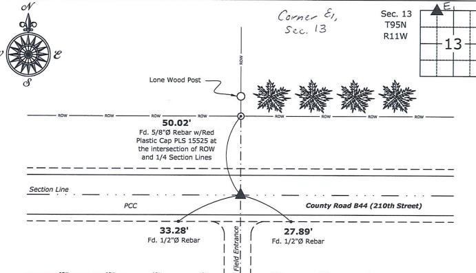
Northeast Corner of the NW 1/4-NW 1/4 of Section 13-95-11 Set 1"Ø Bronze Survey Marker PLS 19211
