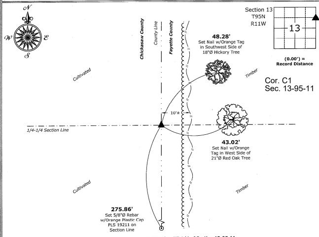
Southeast Corner of the NE 1/4 - NE 1/4 of Section 13-95-11 Set 5/8"Ø Rebar w/2"Ø Aluminum Cap PLS 19211 (Buried 18" Deep)
