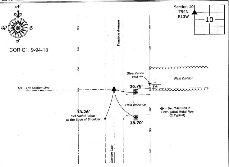
Northwest Corner of the SW 1/4 - NW 1/4 of Section 10-94-13 Set 5/8"Ø Rebar w/2"Ø Aluminum Cap PLS 19211
