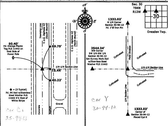
1.) Northwest Corner SW 1/4-NW 1/4 Section 30-94-12 Set Survey Mark Nail w/Stainless Steel Washer PLS 15525
