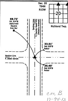
1.) North 1/4 Corner Section 20-94-13 Fd. 3/8"Ø Bolt with Nut
